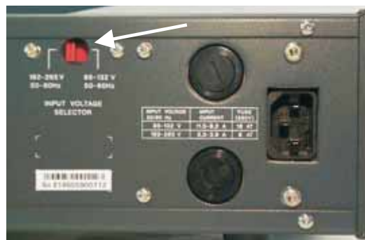
fig. 3 - 2 Input voltage selector at rear panel
