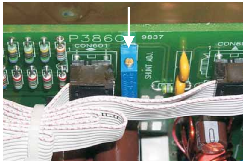
fig. 4 - 24 Calibrating max current P385, P386 or P387
