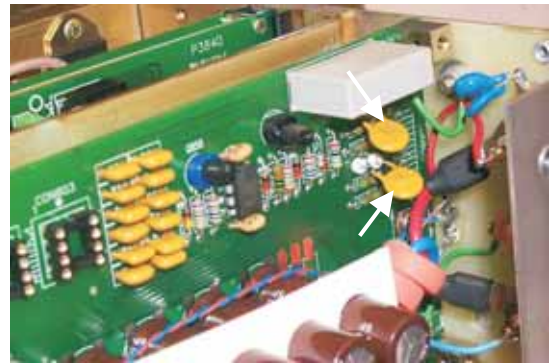
fig. 4 - 18 Location of programming fuses on output board P385, P386 or P387.
