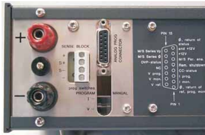
fig. 3 - 10 Location of output terminals, Sense Block, analog prog. connector and PROG. / MAN. switches on rear panel (SM3004-D has no sense block).
